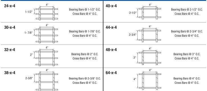
Each product is available in steel, aluminum, or stainless steel, assembled by any of the manufacturing methods presented on this website. To specify the appropriate material and manufacturing method, replace the "x" in the above part number with any of the following designations:
